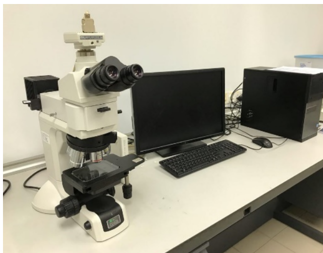
Figure 3 A digital microscope, Nikon Eclipse LV150N, for observing the microplastics.
