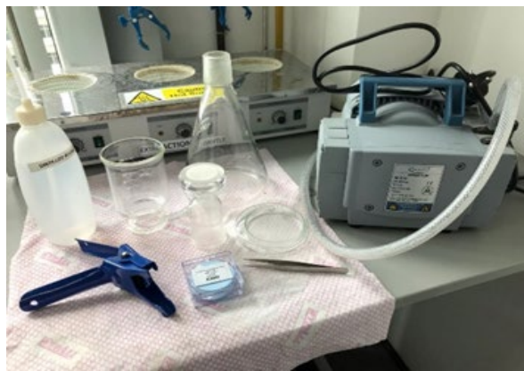
Figure 2 Vacuum filtration setup for the bottled water samples.
