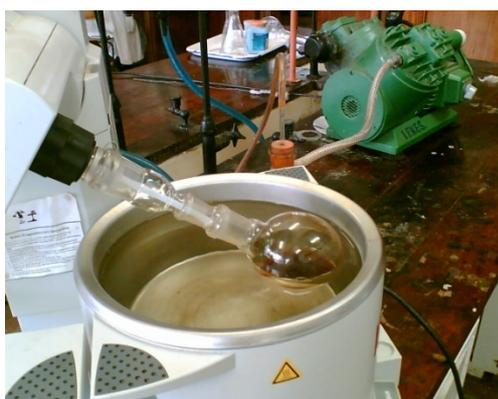
**Fig 16:** Solvent removed from extract in rotary evaporator
